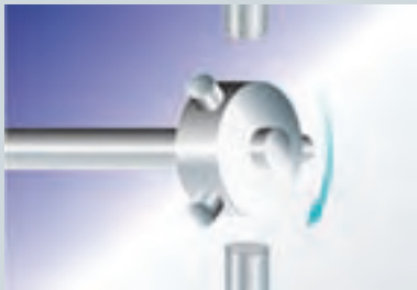
Recognition of positioning screws on the wheel for velocity or direction control
